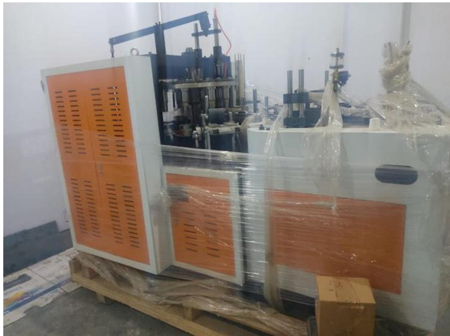
**GI-D paper cup machine** is improved based on the normal chain driving type. This machine runs a whole procedure of paper-feeding, cup-fan-wall sealing, oiling, and bottom punching, heating, rolling, rimming, rounding and tripping. It is idea equipment for producing drinking cups, market cups, coffee cups, advertising cups, etc. It is widely used for hot drink and beverage.
