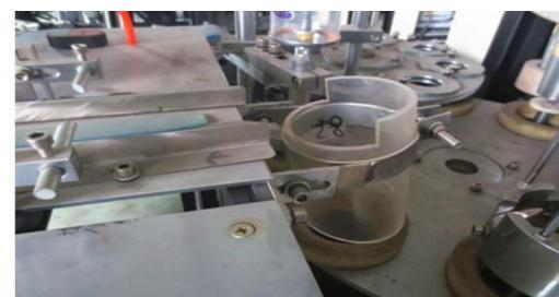
9. Change the Ø25 normal steel shaft to Ø30 imported steel shaft to be strengthened, longer life and more stable.
